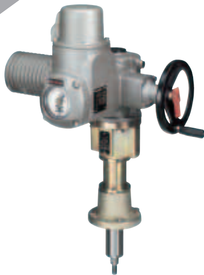
Linear thrust units LE with multi-turn actuators SA Thrusts from 4 kN to 217 kN Strokes up to 500 mm Linear speeds from 20 to 360 mm/min
